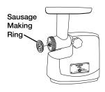
Insert sausage-making ring into feed screw. Make sure notch on sausage making ring aligns with notch in feed screw.
